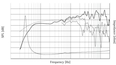
The frequency responses above show measured free field sound pressure in 0, 30, and 60 degrees angle using a 60 L closed box. Input 2.83 YEMS, microphone distance 0.5m, normalized to SPL 1m.The dotted line is a calculated response in infinite baffle based on the parameters given for this specific driver. The impedance is measured in free air without baffle using a 2V sine signal.
