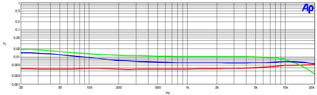
From top to bottom: 40W, 10W, 1WFrequency Response (4Ù, 8Ù and open circuit)
