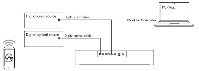
These methods of playing music from the DM35 involve connecting the source to the DM35 via a cable, and don't require Wi-Fi, Ethernet, or Bluetooth.
